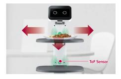
The front, left, and right sides are open to conveniently serve dishes and trays. Each shelf features a ToF sensor that automatically detects food; once removed, the robot automatically proceeds to the next destination, without any additional input required.
