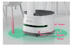
The 3D camera sensor detects low obstacles, while ToF sensors reliably recognize nearby or rapidly approaching objects, allowing ServeBot to avoid even small obstacles as it safely and autonomously navigates the spaces.
