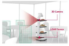
Like the human eye, the 3D camera and LiDAR sensor recognize objects and determine the robot's path, allowing it to freely and accurately navigate, even through (or in) tall, narrow, or complex spaces. Requires advance mapping of table layout for service area.
